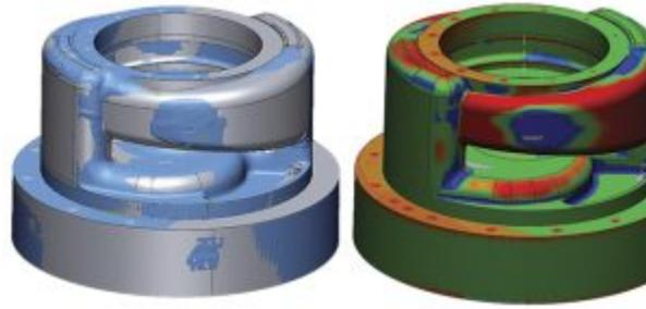
To perform the verification of the casting geometry, a further 3-D scan is taken from the casting. This scan is then compared with the 3-D model and the initial casting scan, and a deviation analysis is performed to ensure that the passage shapes are correct and that there is sufficient machine stock on the casting.
