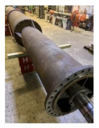
Hydro's Performance Test Lab is equipped with state-of-the-art instruments for testing and has an extensive quality assurance program to support the nuclear industry. The Test Lab provided testing services for the Condensate bowl assembly with its in-house discharge head and motor. This method results in less set-up time and piping fabrication but still assures the integrity of the test.
