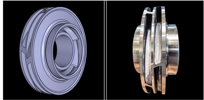
To reduce the pressure pulsation without adversely impacting the machine's hydraulic performance, Hydro designed and installed staggered and raked vanes to the impeller. This required a center rib to be designed into the impeller around which the impeller vanes can be staggered.
