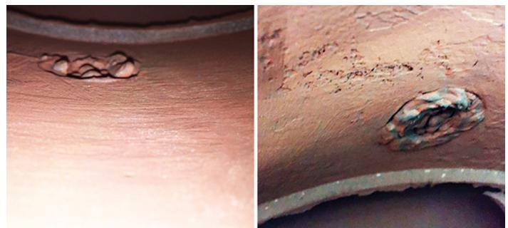
Chaplets are usually comprised of different metallurgy from the metal being poured and can create a weak area if left in place. Image 2 shows areas that were either utilized for chaplets or are core sand clean-out plugs, which were excavated and welded.
