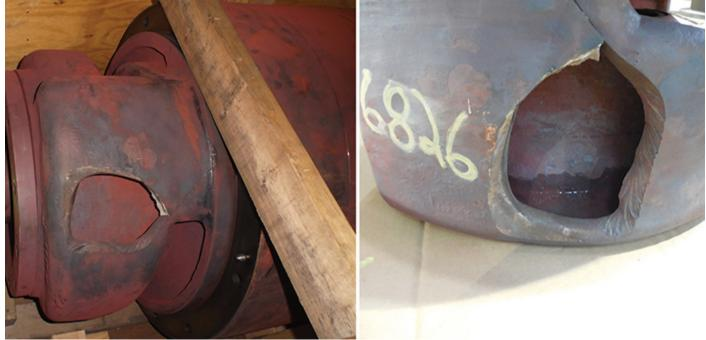
The first-stage twin volute is a complicated casting, which failed during operation as a result of poor design.
