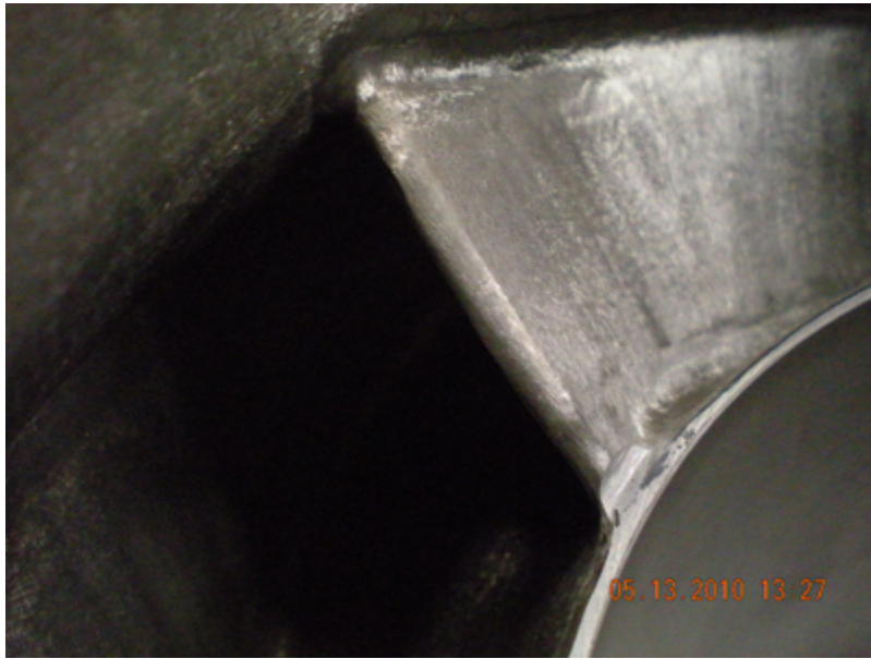
Properly dressed impeller vane.
