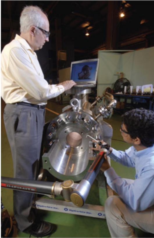
Hydro inspects casing manufactured for a nuclear charging pump. (Photograph by Stephen J. Carrera, used courtesy of Hydro, Inc.)
